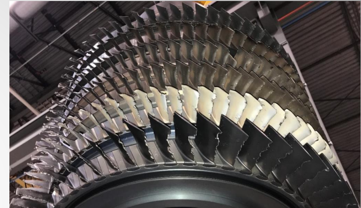
HPC Stage 1 -6 Blade Condition
