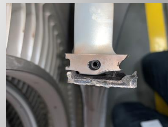
Stage 6 shroud condition at split line
