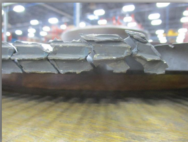
IP Turbine Condition As Found
