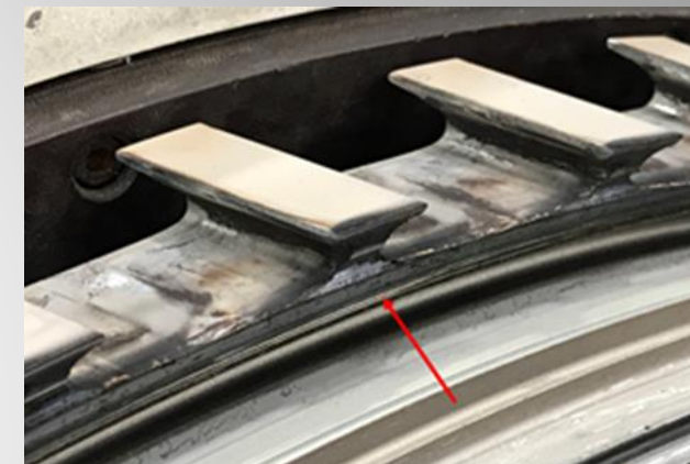
Heavy Rub on aft face of IPC stage 6 Disc Rim
