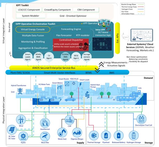
Sets up a virtual network of decentralized, a) vRES generating units such as wind, solar, tidal resources, and b) dispatchable ones, such as geothermal and **green gas** (clean biogas) CHP plants, as well as c) Energy Storage Systems (ESS), integrated as a single unit, providing flexibility services and fostering island REC's self-consumption;
