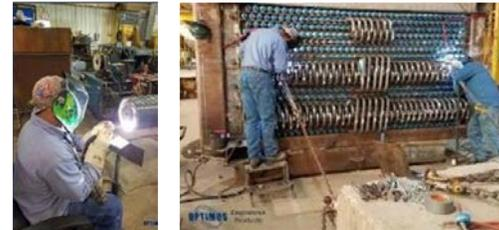
**Heater coil operates at 265 bar and 700°C**
