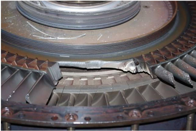
Figure 9 – Catastrophic failure of HP turbine blades
