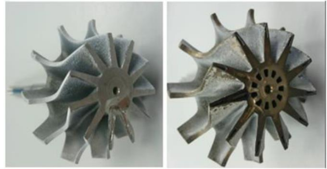
Figure 10: THP coated solid and cooled turbine wheels [2]
