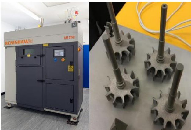
Figure 7: AM250 machine used to manufacture the turbine wheels and manufactured wheels on base plate
