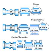
Figure 3 Layout options when VFD is used in LNG refrigeration GT driven trains
