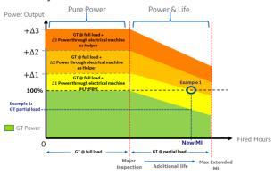
Figure 2 Power augmentation and life extension synergy
