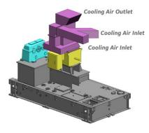
Figure 7 EM air cooling system
